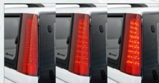
Rear Pillar LED Red acrylic lens with LED Super bright dim and brake light.
